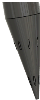
Figure 8: Resin Nozzle Configuration/Spike Penetration Tip
